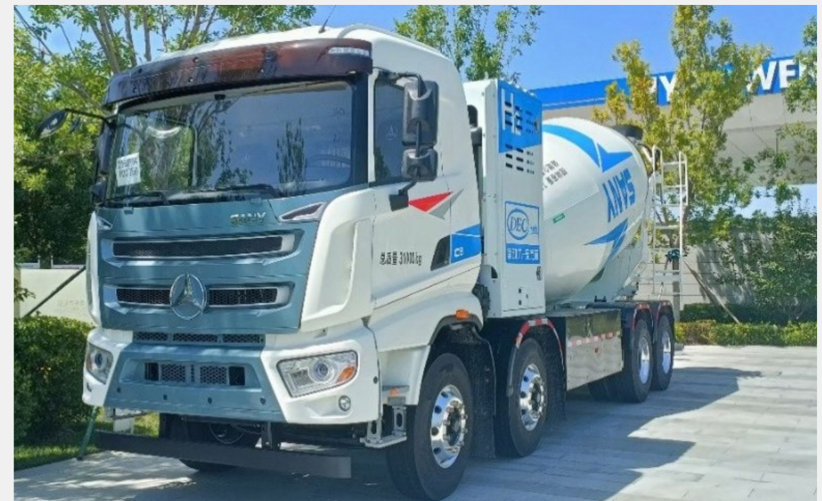
Hydrogen fuel mixer truck
