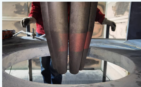
Electric arc furnace developed using long-life graphite electrodes
