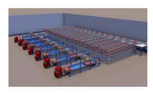
长沙院铜片极板存储及转运系统 Copper sheet electrode storage and transfer system of CINF
