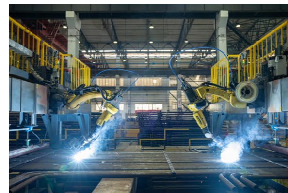
▲自主研发蛇形管附件焊接机器人系统、行业首台大型高压容器全自动激光封口焊上线，锅炉集箱高速数控钻成功实现“双机合璧” The self-developed coiled pipe fitting welding robot system and industry's first full-auto laser sealing and welding machine for large-sized HP vessels form an immaculate pair with high-speed CNC drilling machine for boiler containers
