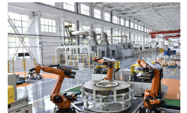
▲定子冲片“无人车间” "Unattended workshop" for stator punching
