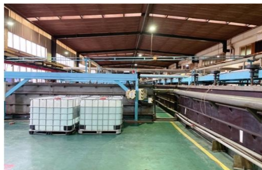
Process optimization and energy saving project of extraction production line: after the implementation of the project, the use of a 142-stage extraction tank will be canceled, 30 motors will be reduced, about 65,000 kWh of electric energy will be saved, and about 46 tons of carbon dioxide emissions will be reduced.
